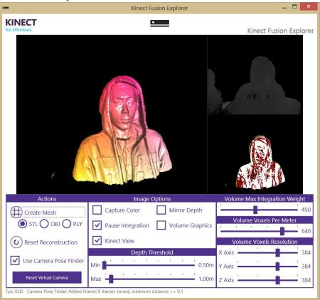
KinectFusion creates a 3D construction with a voxel (3D pixels) representation the reconstruction (which can be converted to various file formats). An in-depth explanation of the parameters can be found at <a href="https://msdn.microsoft.com/en-us/library/dn188670.aspx">https://msdn.microsoft.com/en-us/library/dn188670.aspx</a> and below is an overview of some important information.
